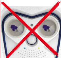
M15 with two transport plugs: No operation allowed!
